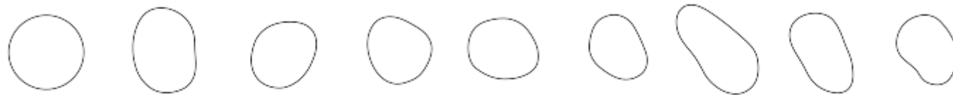
Figure 1: Droplet deformation in a turbulent flow. From left to right the evolution of a single droplet.
