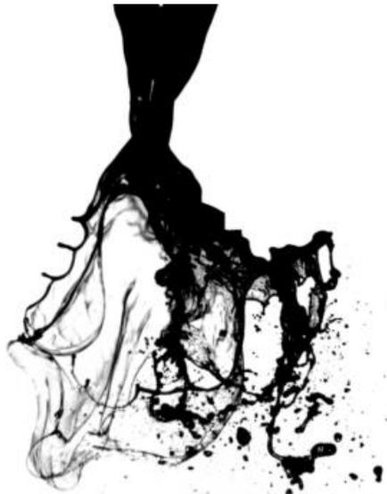
Rims produce large drops that contain a large portion of the liquid volume
