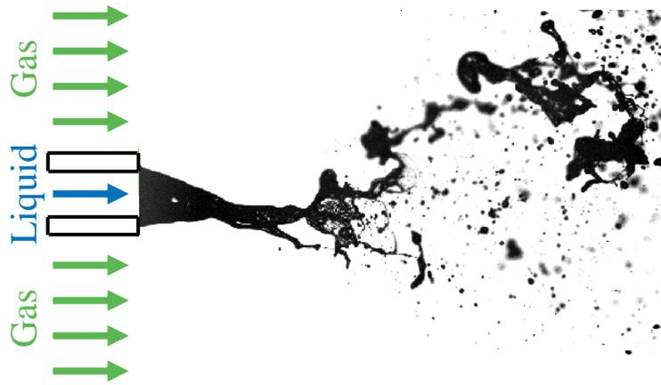
$$We = \frac{\text{gas - induced stresses}}{\text{surface tension}}$$
