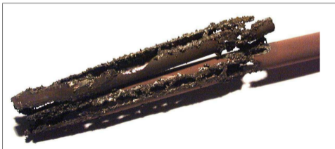
Boiling crisis on heated rods - ©CEA
