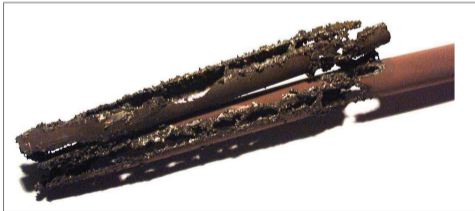
Boiling crisis on heated rods - ©CEA
