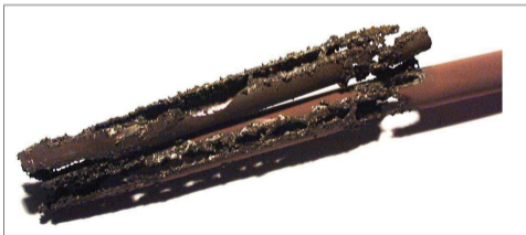
Boiling crisis on heated rods - ©CEA
